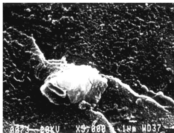
Figure 7 SEM micrograph of a fracture surface of an LCP/PC system showing not very well-defined interfaces between an LCP particle and the PC matrix.
